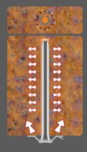
The installed ViDEX<sup>™</sup> friction-bolt exerts radial pressure against the borehole wall over its full contact length, while the washer plate provides load support of the lower section of the ground.
