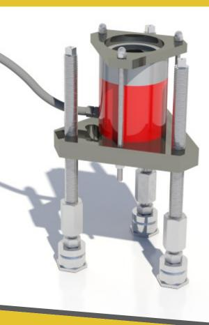
Complete pull-out test system for ViDEX<sup>™</sup> friction bolts is available comprised of a hollow hydraulic cylinder, a hydraulic pump, a manometer for monitoring the applied load, a cylinder resting base and suitable gripping device.
